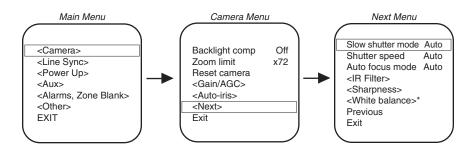
Slow shutter mode slows the frame rate, producing a digital color picture sensitive to low light conditions. The picture may appear rough or smeared, depending on the distance and motion of the viewed image.
